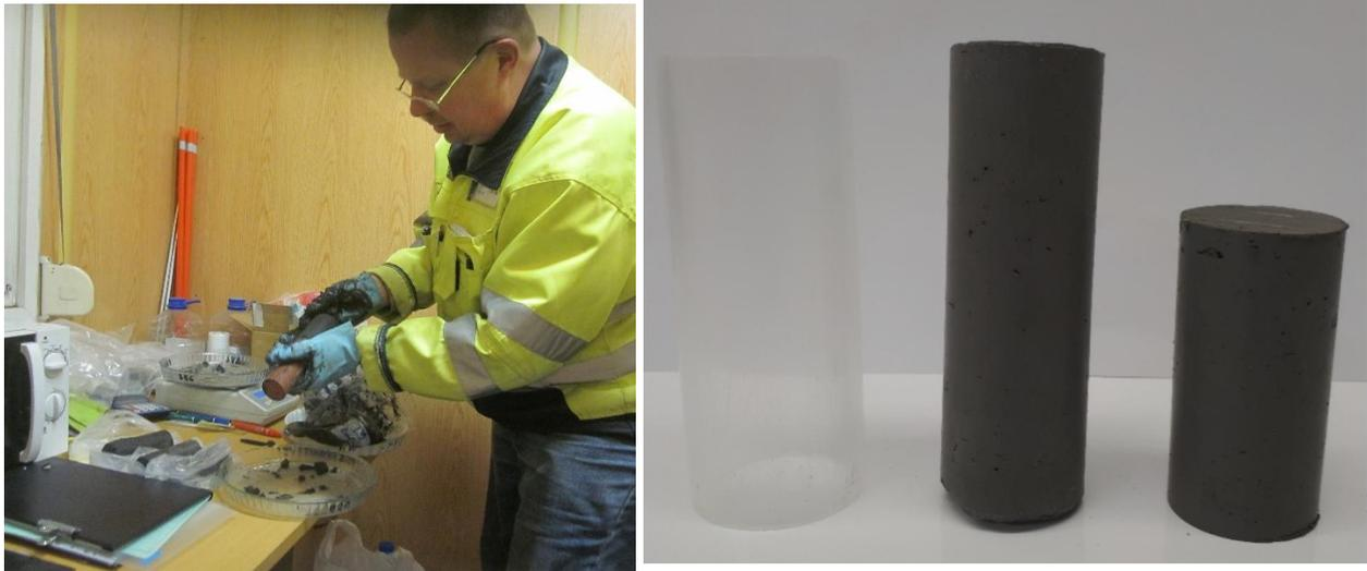
Figure 8. Making of test specimens (left) and after curing time compression strength test specimen is removed from the form, ends are flattened, and specimen is ready to be tested (right).
