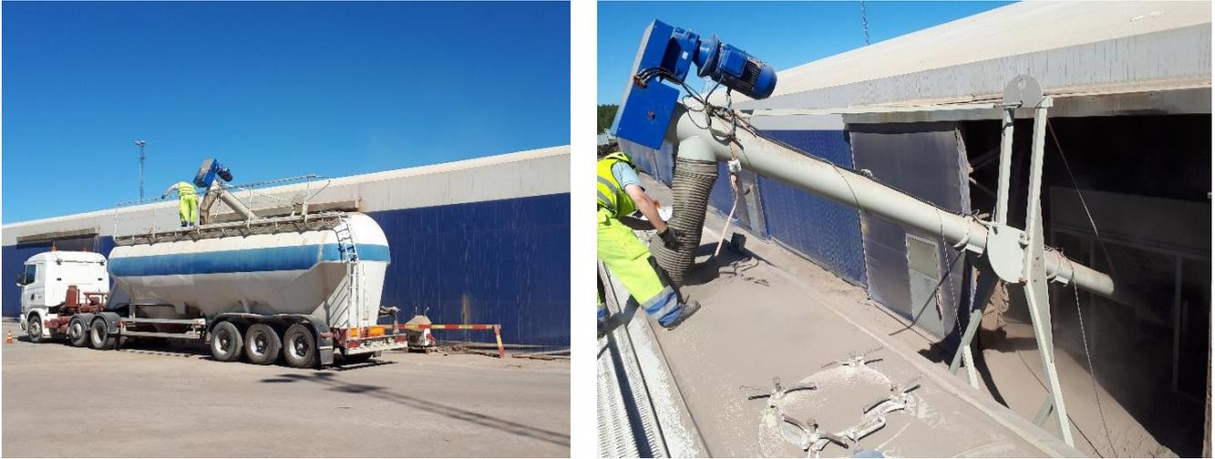
Figure 11. Tarpaulin lightweight hall can be used for dry storage of fly ash from the power plant. Dry ash is stored in hall, loaded to tank truck and transported to stabilization site.
