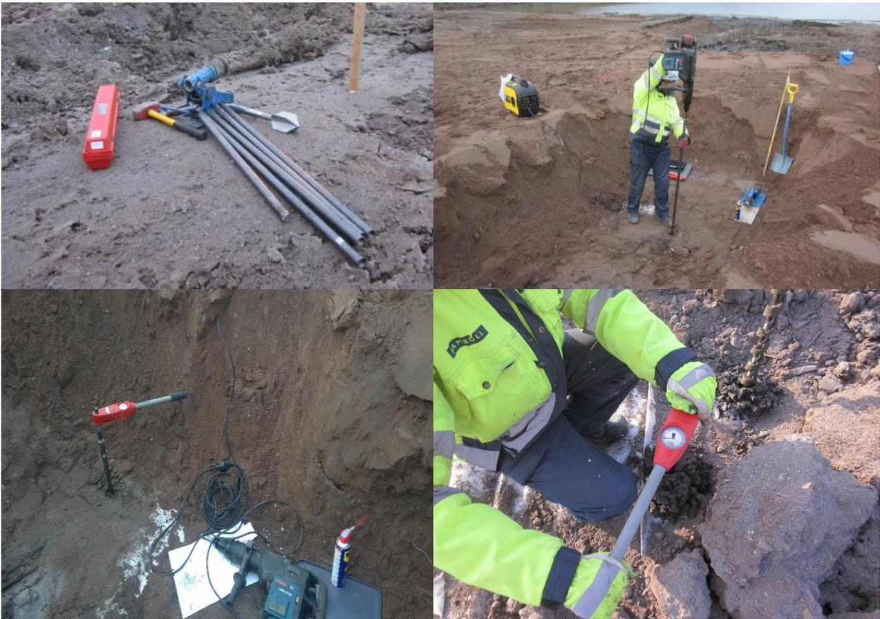
Figure 9. Field inspection vane borer set (top left), vane borer driven down into the stabilized mass to the desired depth (top right) and measuring the shear strength of stabilized mass at the Sampaanala bay (bottom left & right).
