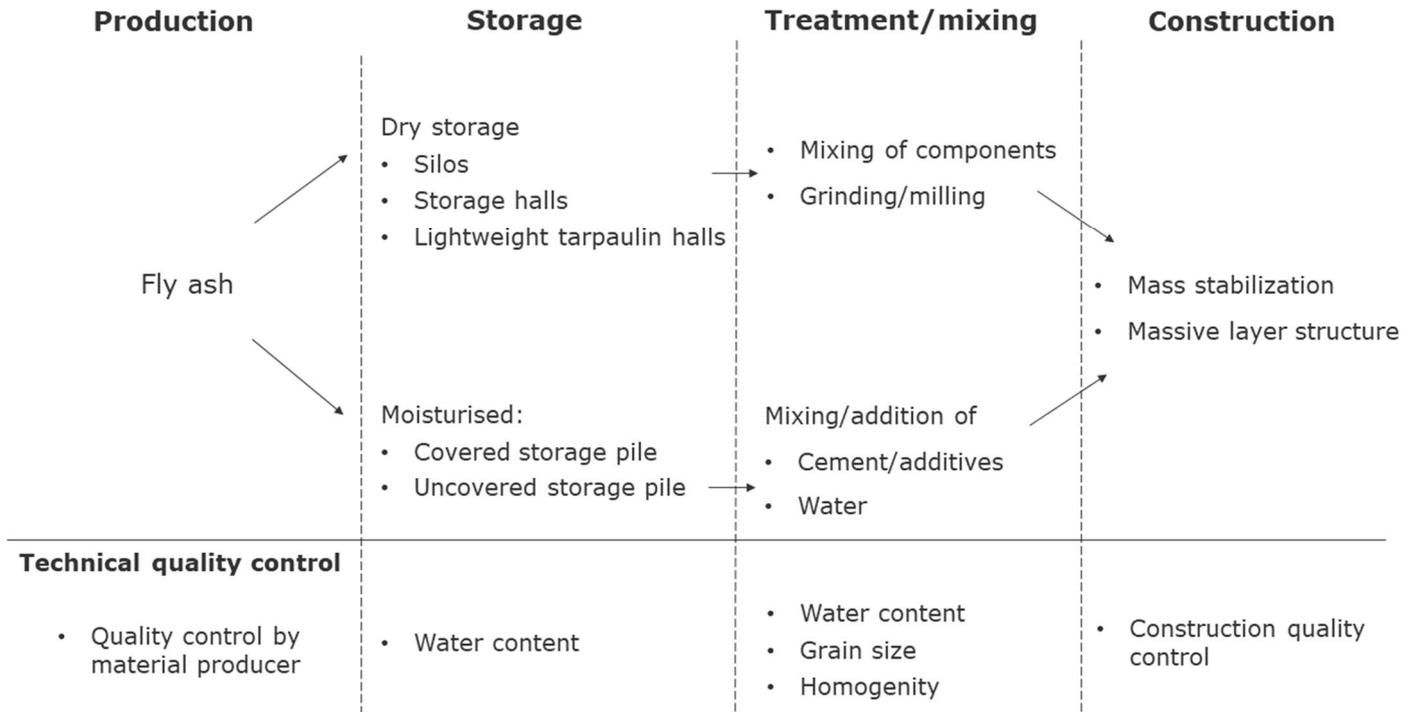
Figure 13. Brief summary of fly ash technical quality assurance during each phase in construction project
