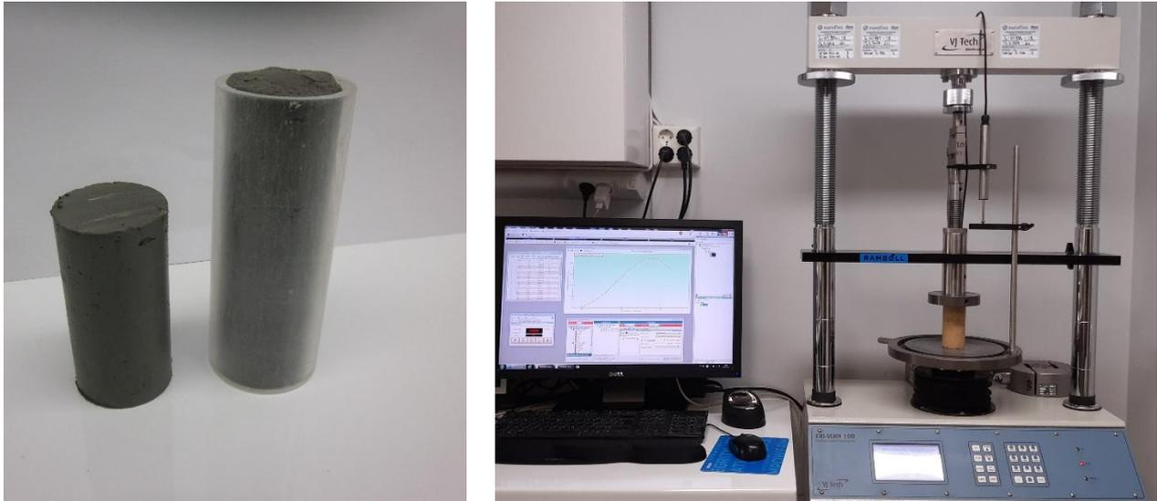
Figure 2. Stabilized test specimen (left) and UCS testing equipment (right)
